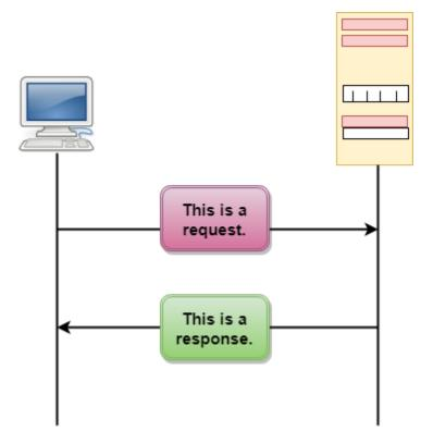
The above figure shows the HTTP transaction between client and server. The client initiates a transaction by sending a request message to the server. The server replies to the request message by sending a response message.
