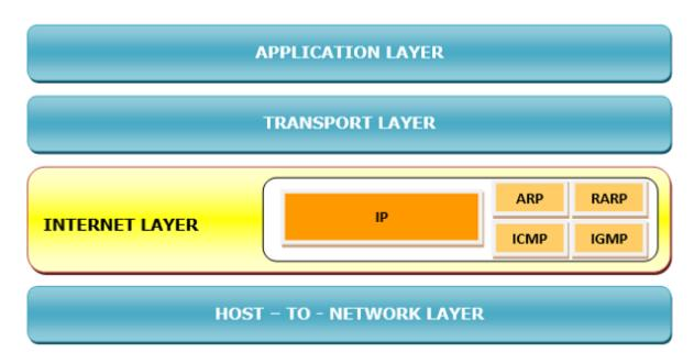
The following diagram shows the network layer in the TCP/IP protocol suite -
